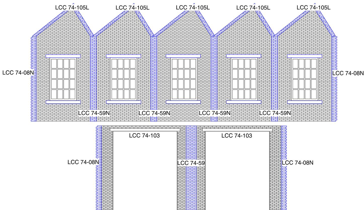
Using the diagram above glue all of the decoration parts to the walls. Note that LCC 74-105L should be glued to LCC 74-104L and LCC 74-105R should be glued to 74-104R.
