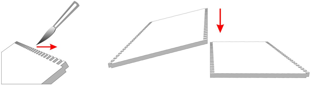
Recommended way of gluing parts together is to apply PVA glue to the interlocking bricks working from back of the part to the front. This ensures there will be no glue overflow on the front, visible side.
